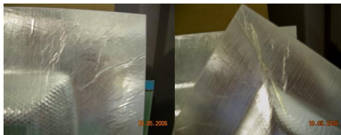
Figure 4: Wrinkling Formation on Sandwich Panels
